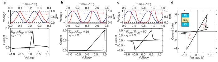
**Figure 3** | **Simulations of a voltage-driven memristive device. a**, Simulation with dynamic negative differential resistance; **b**, simulation with no dynamic negative differential resistance; **c**, simulation governed by nonlinear ionic drift. In the upper plots of **a**, **b** and **c** we plot the voltage stimulus (blue) and the corresponding change in the normalized state variable *w/D* (red), versus
